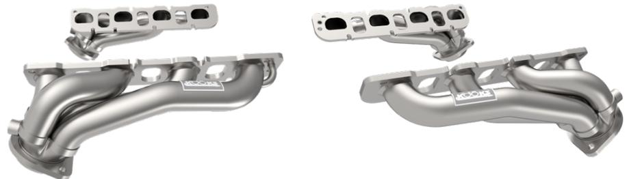
With the Super Street Series headers equipped on the 5.7L HEMI engine, the dyno test results produced gains in both horsepower and torque without tuning. The dyno graph presented an increase of 19 horsepower and 23 lb-ft of torque over the stock manifolds when measured at the tire. Performance gains may vary depending on tuning and other performance modifications.
